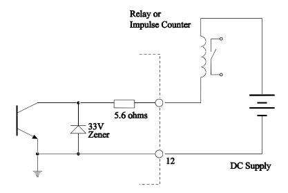
Driving an External Relay or Impulse Counter
